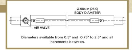
Three Continuous Grip Ledges on 1" Diameter Shafts and Up
